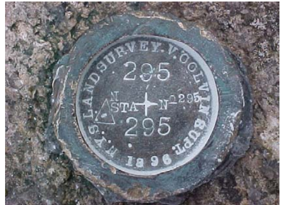
One of Colvin's last known points, Bolt 295 set in 1896 on Eagle Island
