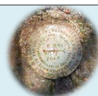
U.S.C.&G.S. Crown Point North (1943) Reference disc No. 1 in exposed bedrock – 85' from station.
